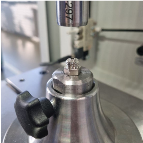
Image 2: Round-head brass grease nipple, operation: flanging with stroke and force measurement
