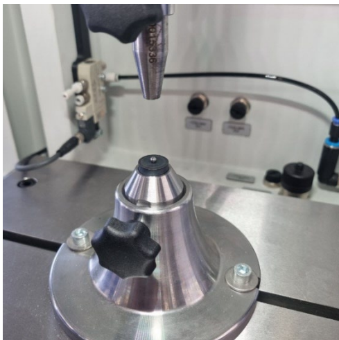
Image 3: Valve seat N1 , operation: valve seat with force measurement
