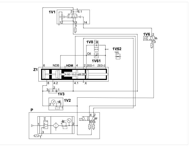
The damping is set on the flow control valve (1V61 or 1V62). The electrically switchable solenoid valve (1V8) makes individual activation and deactivation of damping possible. With the standard stroke monitoring on the working piston the time can be specified at which damping is to be activated.
