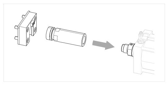
Fig. 28 Installing tool coupling (ZWK)
