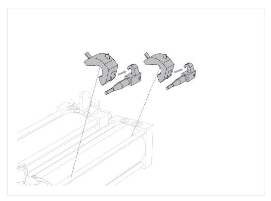
Fig. 19 Installing position sensors for stroke monitoring for forward and return stroke
