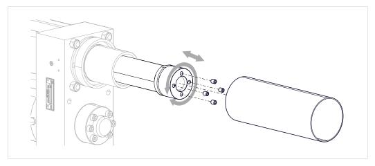
Fig. 32 Setting total length of stroke
