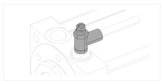
Fig. 29 Setting control throttle 'X'
