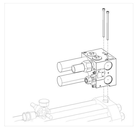
Fig. 26 Installing the stroke frequency optimization ZHO
