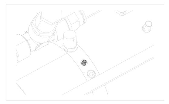
Fig. 36 Checking oil level
