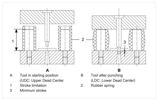
Fig. 15 Stroke limitation in the tool
