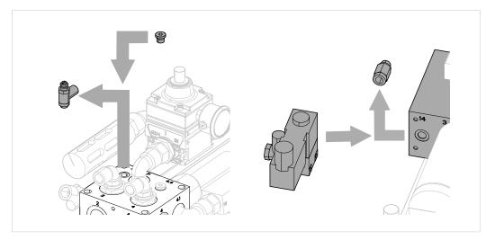
Fig. 22 Installing external power stroke connection (ZKHZ)
