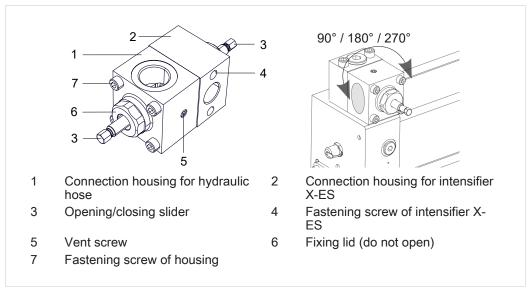
Fig. 12 Hydrosplit coupling ZHK, manually switchable
