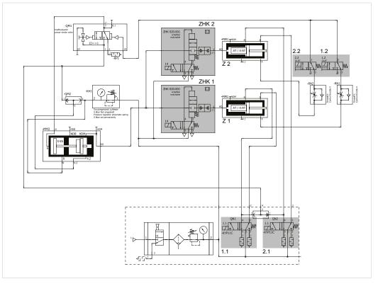
Fig. 30 Control plan X-AT, AT hydrosplit coupling ZHK
