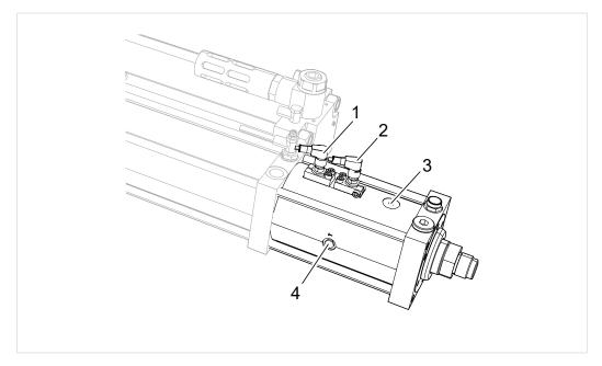
Fig. 34 Setting the proximity sensors of the holding brake
