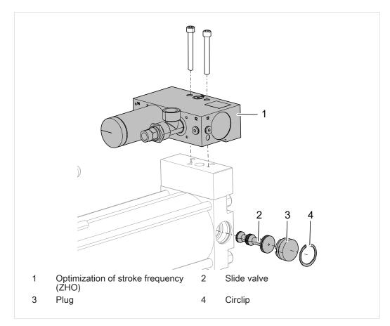
Fig. 25 Installing the stroke frequency optimization ZHO
