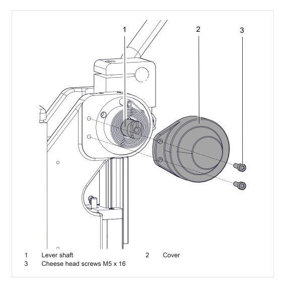
1. Unscrew the lever shaft from the cover. The flat spiral spring must nor be removed.
