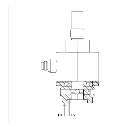
→ NOTE! Observe the maximum thread length! The tool must bear against flange 1 or flange 2.
