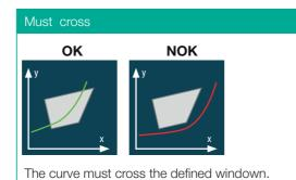
Application: Monitoring of the force-travel progress during pressing in of elements
