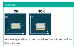
Application: Control of the average force applied to a piece part when clamping, forming or molding.
