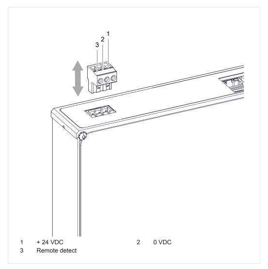
Fig. 3 Supply voltage connection
