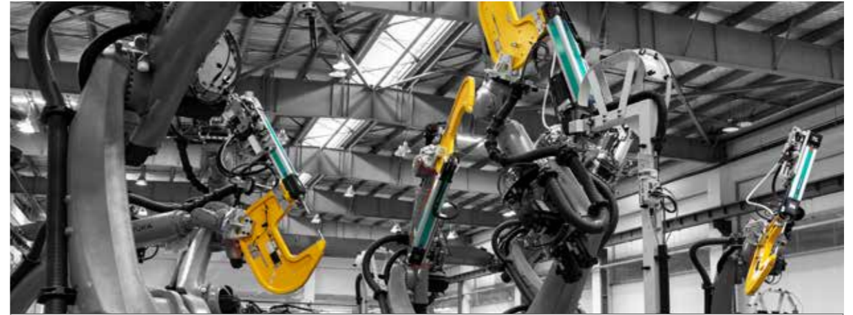
TOX® Riveting System SPR Robot-guided frames in a robotic cell that join car body parts with rivets.
