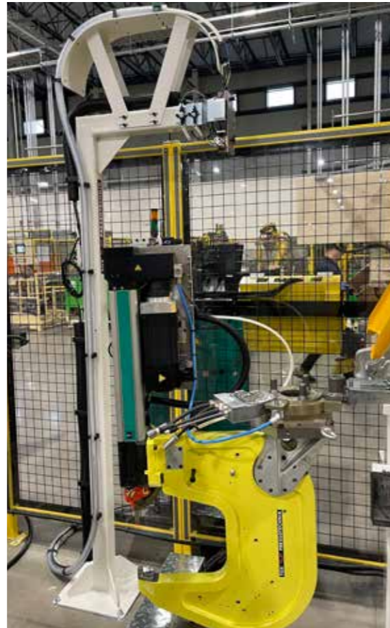
TOX® Riveting System SPR in dock-feed configuration.
