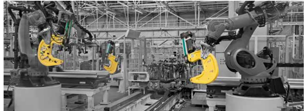
TOX® Clinching System Robot-guided frames in a robotic cell join car body parts.
