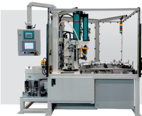
C-Frame Press as a manual workplace. It presses in rivet bolts in a part of a car hood.
