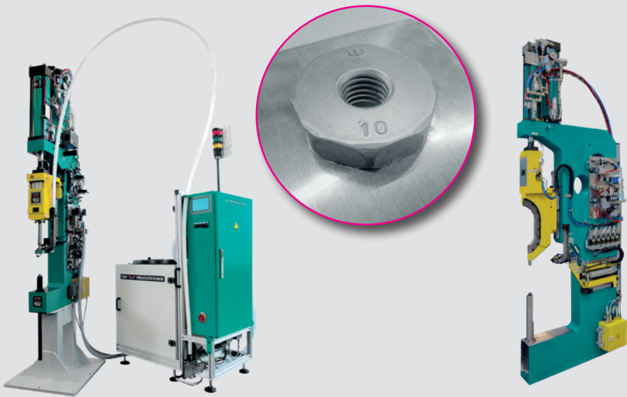
Stationary Tongs for pressing in self piercing nuts.
