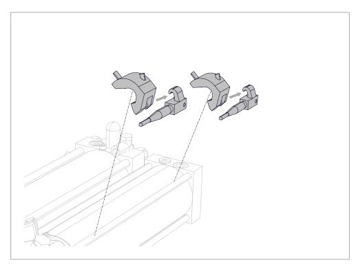
Fig. 2 Installing position sensors for stroke monitoring for forward and return stroke
