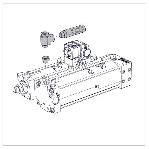
Fig. 7 Installing the speed reduction for power stroke venting
