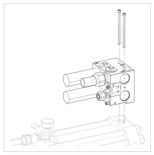
Fig. 6 Installing the stroke frequency optimization ZHO
