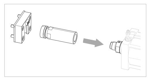
Fig. 8 Installing tool coupling (ZWK)
