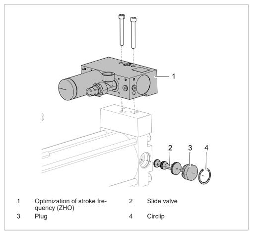
Fig. 5 Installing the stroke frequency optimization ZHO
