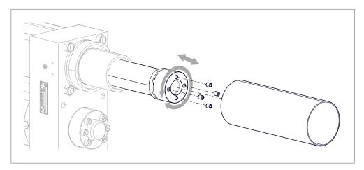
Fig. 10 Setting total length of stroke
