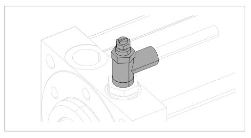
Fig. 9 Setting control throttle 'X'
