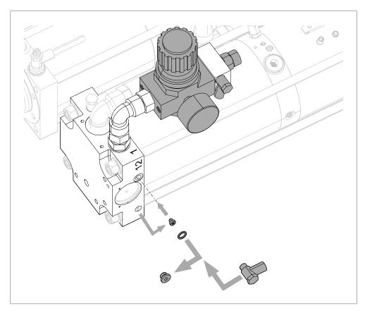
Fig. 3 Installing pressure control in the power stroke line (assembly ZDK)
