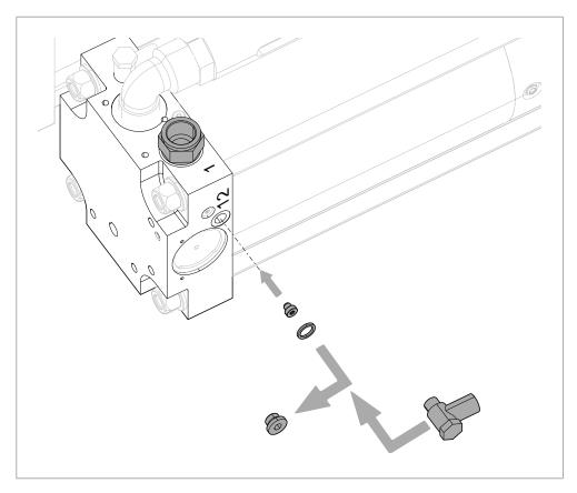
Fig. 4 Preparing external power stroke supply
