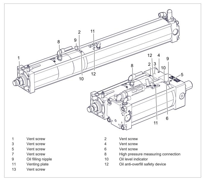
Fig. 12 Refilling oil and venting drive
